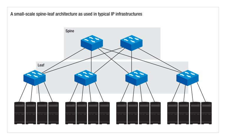
Multiple GV Node IP routing and processing nodes can be readily connected to a COTS switch, using a mix of I/Os to create large and flexible monitoring, switching and processing systems. GV Node can be added to both existing facilities as a "top of rack" expansion, and as a scalable standalone system that can grow as your needs increase, and as new technologies become available.
