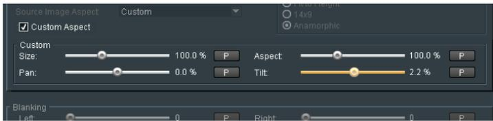
**Note:** as an alternative to using the slider controls, a user can enter specific values for the four controls Size, Asp, Pan and Tilt, by selecting the value parameter and typing a specific value with the keyboard. Alternatively minor step adjustments can be made using the left and right cursors.
