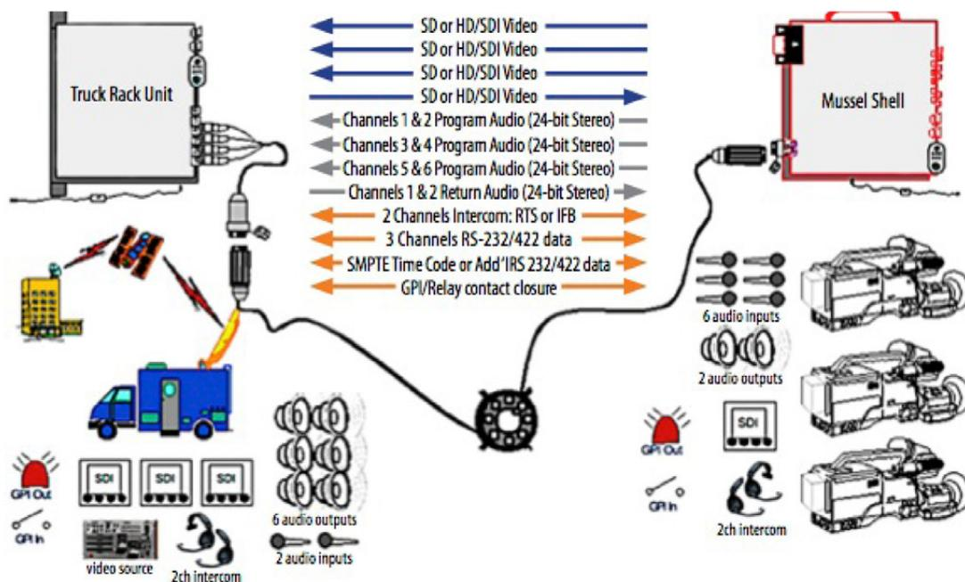
Fiber optic cable can dramatically lower the weight, reduce costs, and allow the multiplexing of various signals through a single, rugged lightweight cable. In many modern sports venues, fiber installations are built-in permanently and use push-pull SC or standard telecomtype ST connectors in a central patching area in the venue. In these cases it is KEY that the fiber infrastructure is properly maintained and managed to insure continued high performance.
