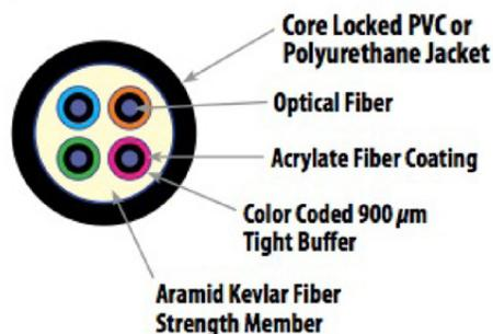
Tac cables are surprisingly flexible, and will not break when the cable is knotted or bent in normal use. As a general rule, one can treat a high-quality Tac cable as a similar sized coaxial cable and it will be very safe. A Tac cable is much more durable, and can routinely be used in much more hostile environments, such as flying cables in temporary self-supporting installations or where vehicle and/or foot traffic is expected.
