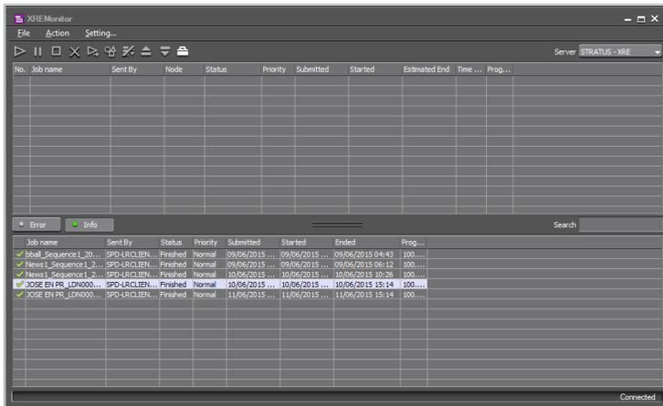
Requesting a rendering job is as simple as selecting “Print to File” from the EDIUS workstation, the file format preset and the destination server. Once the instruction has been sent to the server, you are free to carry on with a new project, removing delays and unwanted bottlenecks.
