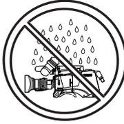
Avoid very damp places. If the environment is wet or damp a rain cover must be used to protect the unit.
