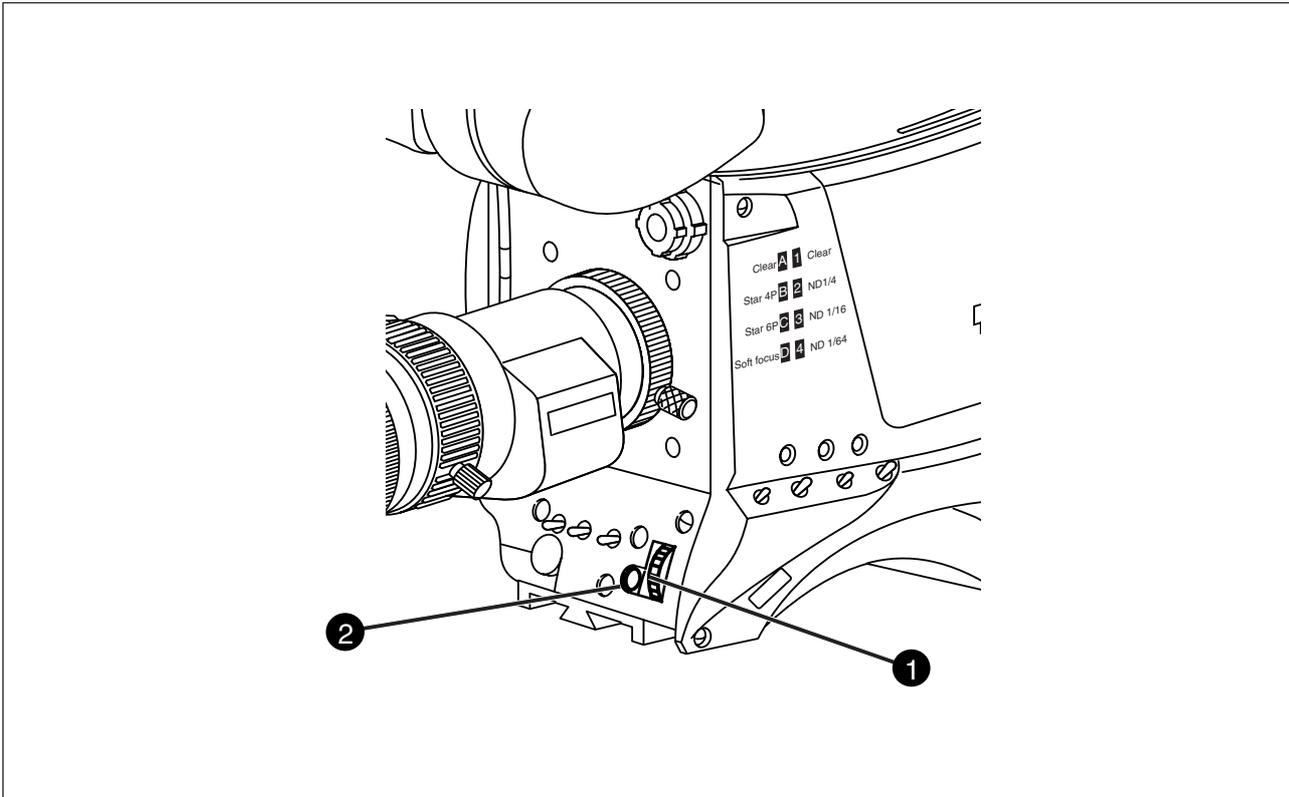
The system menus are displayed in the viewfinder. There are two controls at the front of the camera that allow you to navigate through these menus.
