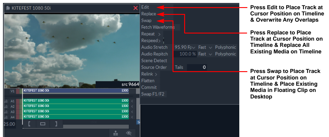
Figure 24 Using Floating Clip More Options Menu to Add Audio to the Timeline
