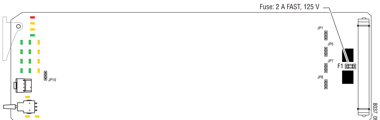
Figure 18. 8920MUX Module Fuse Location
