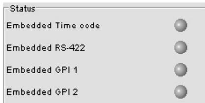
The **Status** tab shows the detection of input embedded time code, RS-422, GPI 1 and GPI 2 signals. When present, the status icons turn to green.
