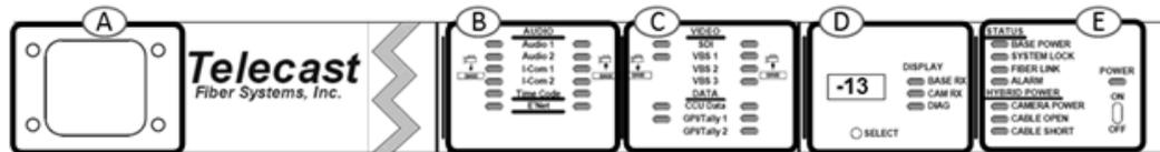
Fig. 3-14: - CopperHead 3200 Base Station Front Panel
