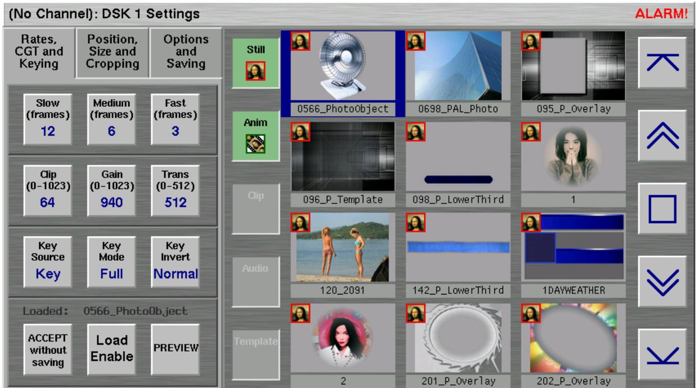
By selecting the appropriate buttons to the left of the image browse area it is possible to choose which types of files to show within the browser. Within the configuration file it is also possible to define the file types that are shown for each of the buttons for each DSK.
