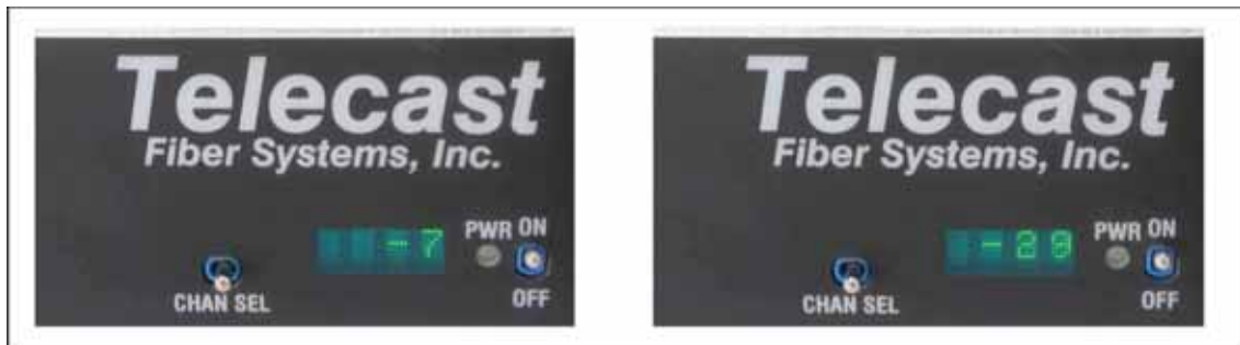
Figure 6 : Variable optical power levels = NO SDI present
