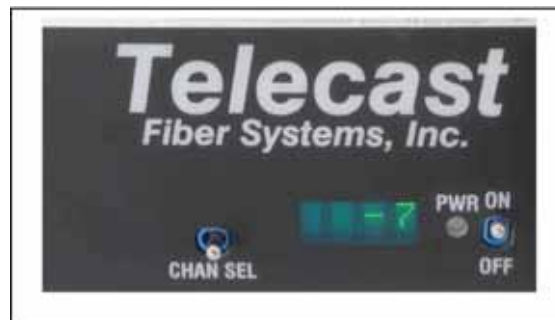
Figure 7 : A steady numerical value IS the received optical power for that channel.
