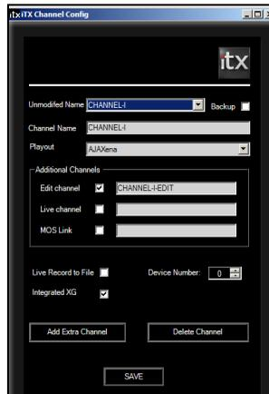
Figure 2-2. Enable the Integrated XG setting
