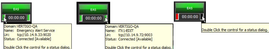
Regardless of the service's or channel's state, you can double-click the status button to display the **Service Provider Status** dialog, which provides even more details. Click the **Run Self Diagnostic** button to run and display a Diagnostic Report.
