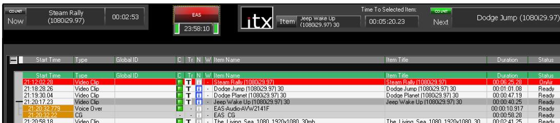
The duration of the CG event is determined by the **Crawl Duration** setting on the **EAS Config** tab, while the Voice Over event's duration is determined by the duration of the audio file from the EAS device. If however, the duration of the audio file from the EAS device is longer than the **Crawl Duration** value, then the audio's duration is used to determine the duration of both the CG event and the voice-over event.
