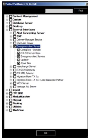
3. Verify the installation by selecting **Start>All Programs>iTX 2.0>Server Controller** to ensure that the Emergency Alert Service is listed on the Server Controller and that the **Emergency Alert Service** window is also open. Select the **Trace Logs** tab and the **Diagnostics** tab to check for any errors.
