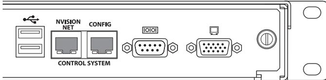
Figure 1. Ethernet Connectors
