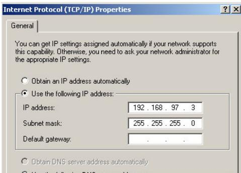
The default IP address of the NV915 on the Config network is 192.168.97.1. Therefore, choose 192.168.97.3 or a similar address that is not the same as the NV915's.
