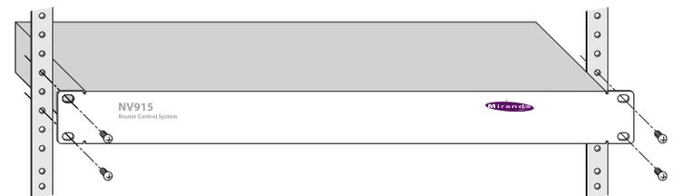
The mounting holes are spaced 1.25" (31mm) vertically and allow approximately 1/8" (3mm) of play horizontally.
