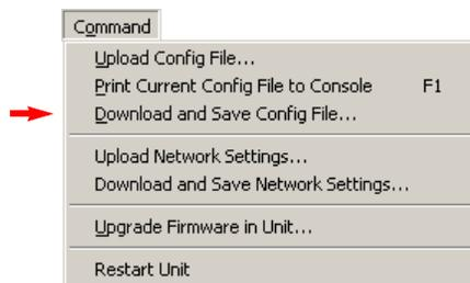
This command copies the configuration from the NV9575-VF to a file in your PC. The file contents appears in the Videoframe Configuration window.
