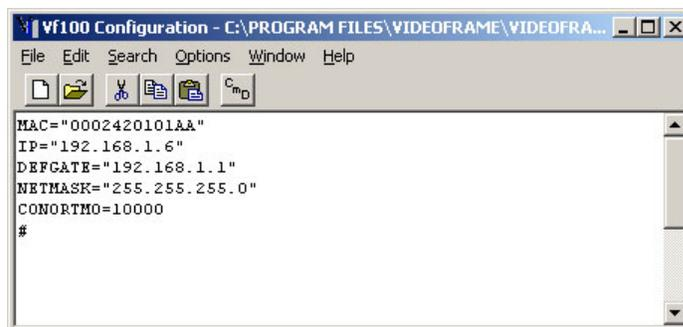
Modify the configuration, in this window, as required. In particular, specify the IP address of the NV9575-VF and ensure that "CONORTMO"—connection override timeout, in milliseconds—is 10,000 or more.
