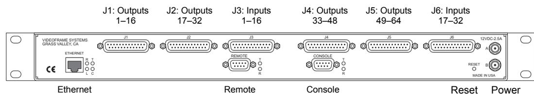
The NV9575-VF has 6 DB25 connectors on its rear panel—J1 through J6. J1, J2, J4, and J5 provide connections for the 64 relay outputs, 16 per connector, with 8 pins common. J3 and J6 provide connections for the 32 inputs, also 16 per connector with 8 pins common.
