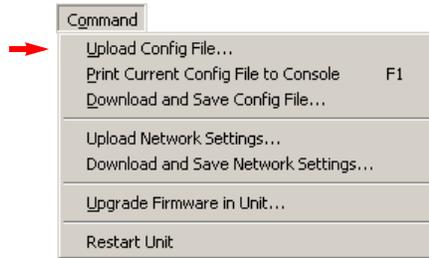
This copies the modified configuration back to the NV9575-VF. The console window displays a confirmation.
