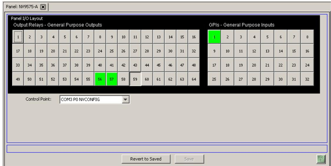
**Note:** The “buttons” you see on the NV9575-VF page represent connections at the rear of the panel. The NV9575-VF has no buttons.
