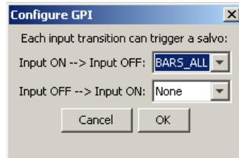
An event is signalled when a transition occurs on the input from on to off or from off to on. You can configure the NV9575-VF to recognize either occurrence on any of the 32 inputs, and specify the salvo to execute at either occurrence or both.
