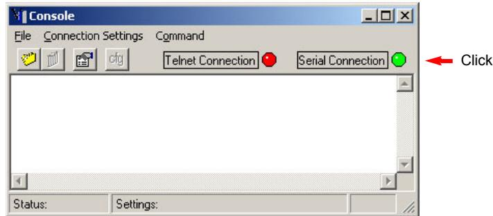
Click the 'Serial Connection' button to make it turn green. This activates serial communication.
