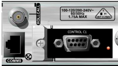
RollCall™ BNC connector on rear of UpCaster Enclosure
