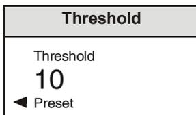
The lowest level of 0 gives the greatest sensitivity to motion, but allows more noise to break through, while 15 gives the greatest noise reduction but can lead to excessive filtering of low-level textures. When this is set to "auto" the threshold is dynamically set to an appropriate value for the current input noise level.
