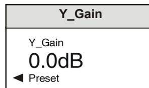
By using the spinwheel the gain may be adjusted by  $\pm 6$  dB in steps of 0.1 dB.
