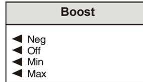
To maximise this effect, the **Max** boost setting is used. It is not necessary to have boost as it can be set to **Off**. A small amount of boost can be obtained by using the **Min** setting.
