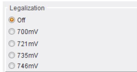
All color video signals are ultimately coded as RGB for display on a picture monitor. The Legalizer ensures that the output video stays within the legal RGB gamut limit, making it suitable for the broadcast signal chain. To achieve this, the Legalizer reduces the gain equally on all channels.
