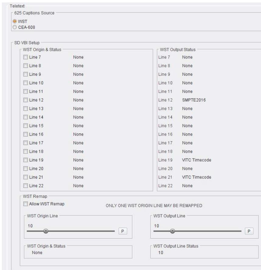
The unit can pass World System Teletext (WST) for SD and RDD-08 or SMPTE 2031 teletext for HD. You can enable or disable teletext output and specify the input and output lines used.
