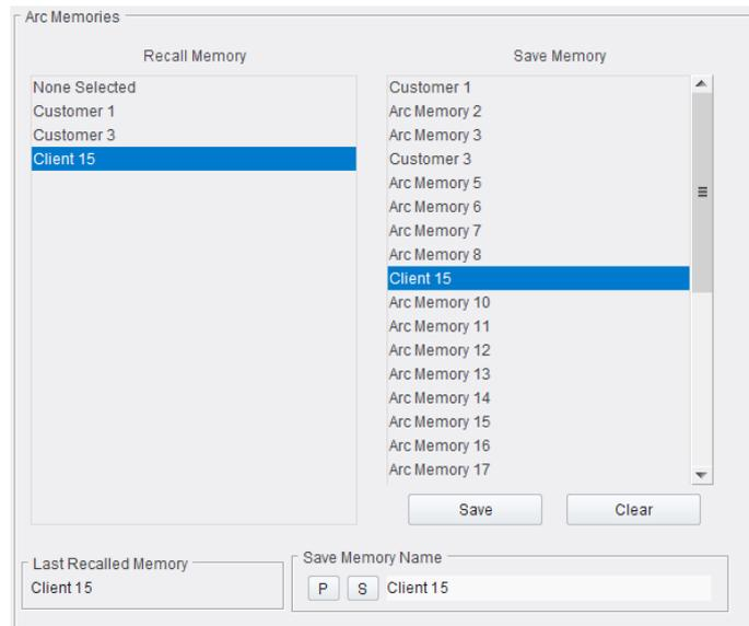
ARC memories allow save and recall of ARC settings, without changing any of the other unit settings. They are useful where specific ARC control needs to be rapidly changed, for example response to signaling, without changing any of the unit input, output, enhancement etc settings. There are 32 ARC memories.
