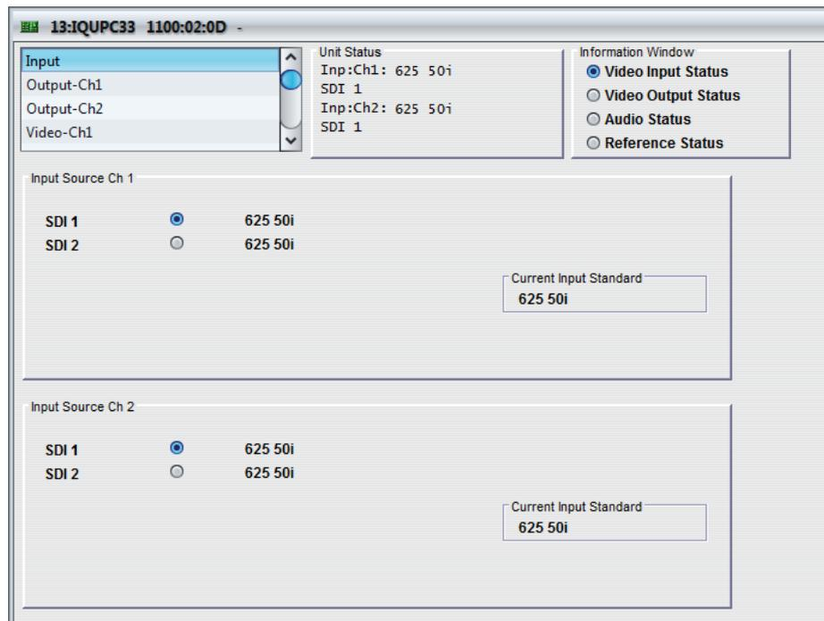
**Note:** The Input Source Ch 2 controls are only applicable to the IQUPC31 and IQUPC33.
