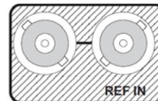
Operation to full specification is only possible with a correctly terminated, noise-free, stable, black sync reference input. While lock may be achieved with an unsuitable sync source, the increased jitter evident on the SDI output will affect locking and cable length performance at the receiving equipment.
