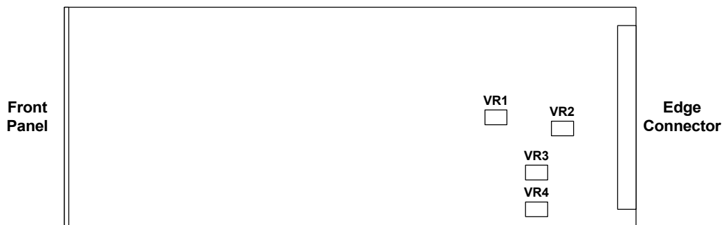
Location of on-board adjustable components
