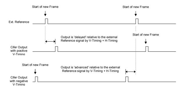
This drawing illustrates the **Reference-to-Output** timing relationship when operating Cifer locked to an external analogue reference.
