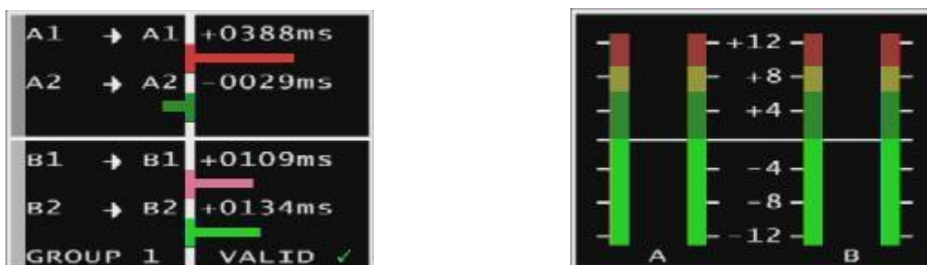
Figure 13 Four Channel Delay Meter and PPM Display
