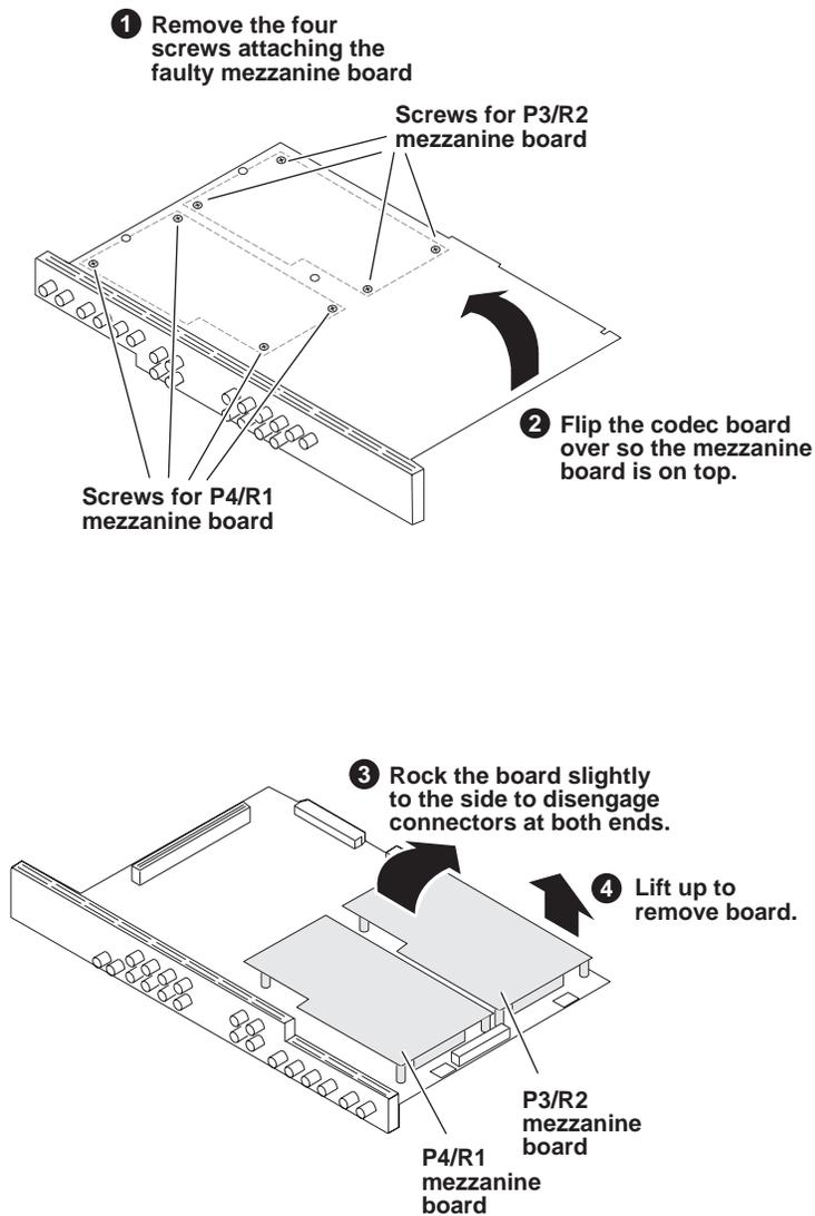
**NOTE:** Make sure the replacement board is the same type (encoder or decoder) and installs in the same position as the faulty board. Changing the type, position, or number of encoder/decoder mezzanine boards renders the K2 Media Client inoperable.
