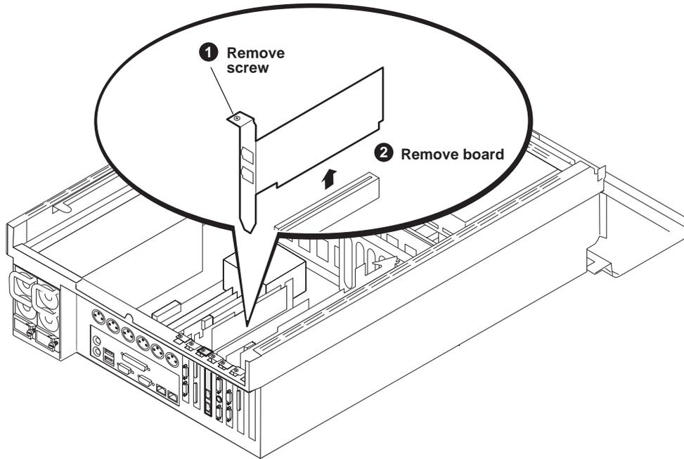
On HD/SD models the Dual Ethernet adapter is in rear panel slot five, as shown. On SD-only models the Dual Ethernet adapter is in rear panel slot two.
