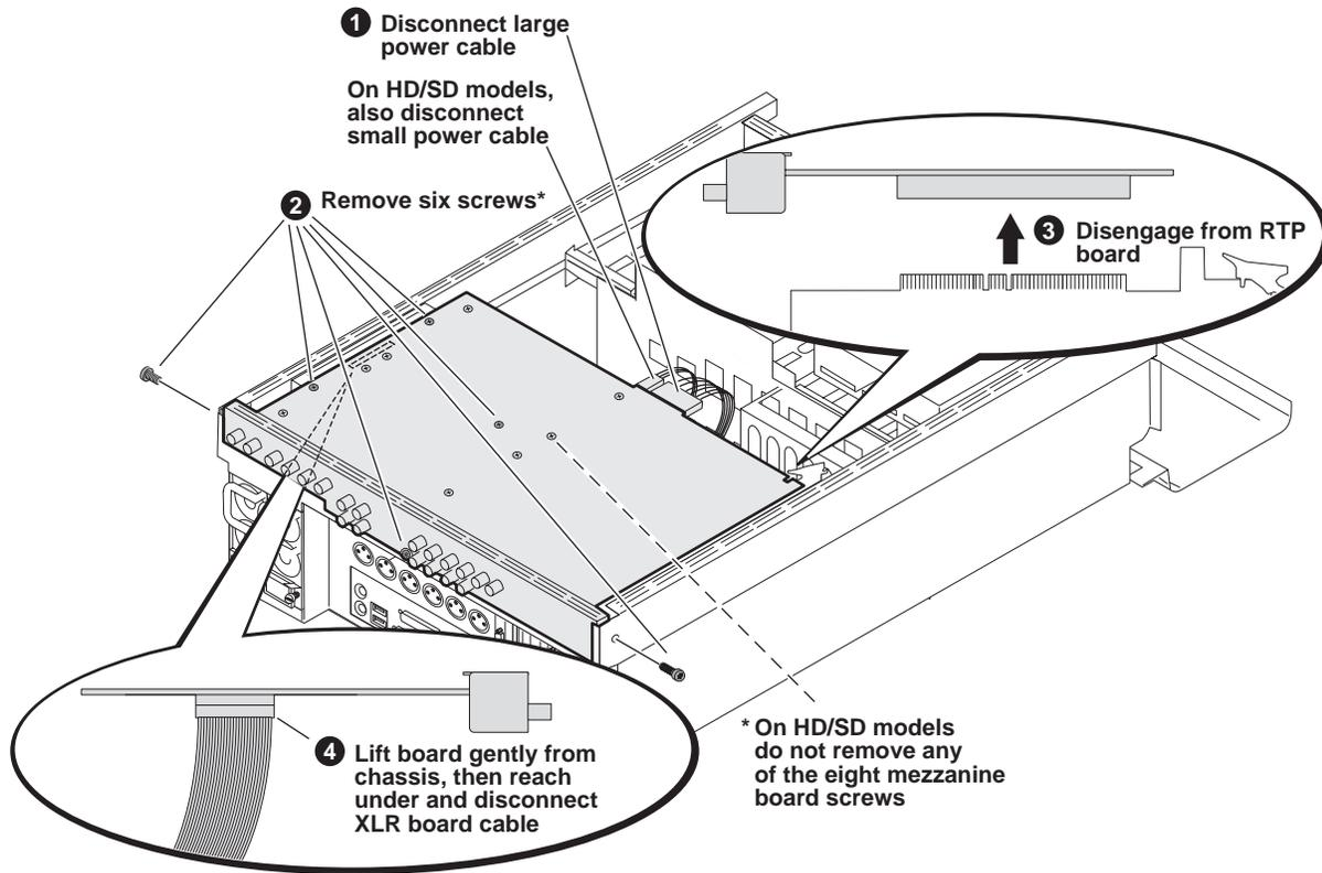
The codec board in HD/SD models and the codec board in SD-only models are different sizes. On HD/SD models the codec board is wider, as shown. This requires that the RTP board be in rear slot two. On SD-only models, the codec board is narrower, which requires that the RTP board be in rear slot five. Take this into consideration when removing a codec board.
