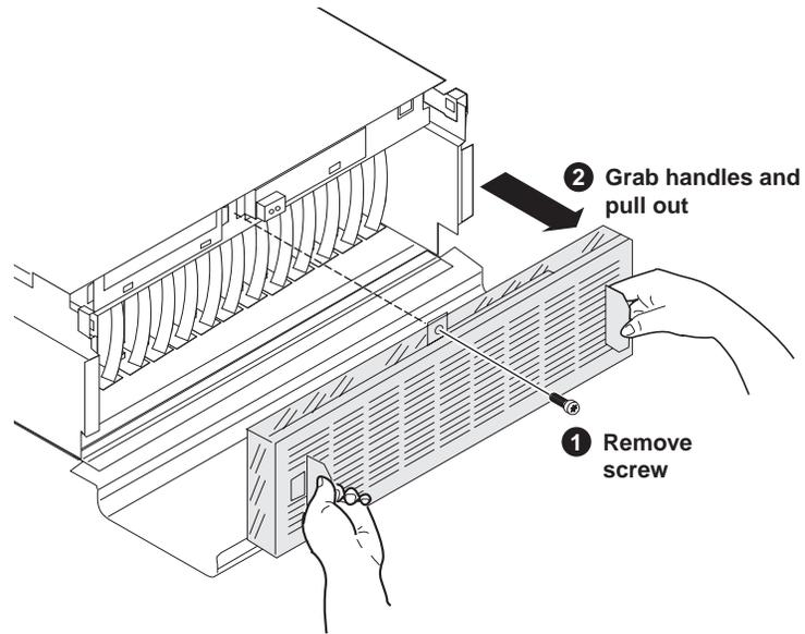
You can remove the fan module while the K2 Media Client is operating. If you do so, make sure you replace it within one minute to ensure that the correct operating temperature is maintained.
