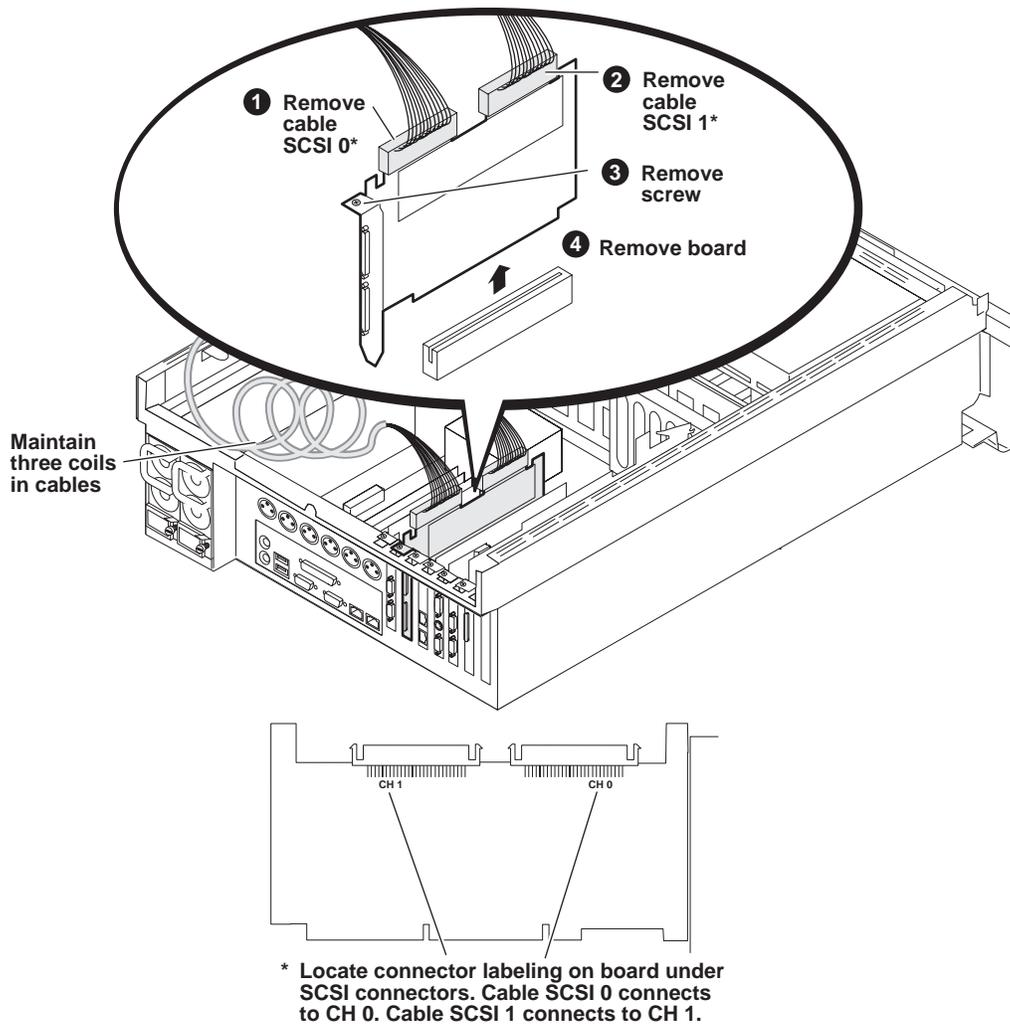
On both HD/SD models and SD-only models the RAID controller adapter is in rear panel slot six, as shown.
