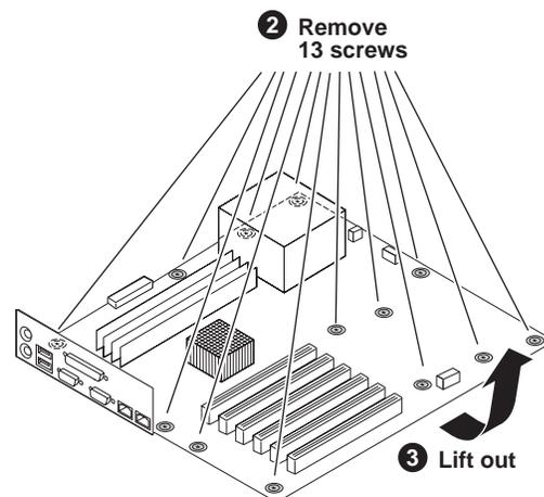
Save the connector panel to exchange with the replacement motherboard. When installing the replacement motherboard, first install the connector panel on the motherboard, being careful to engage flanges on connectors. Then install the motherboard in the chassis, making sure the connector panel “snaps” into the chassis on all edges.
