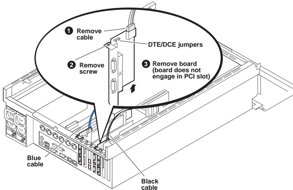
The RS-422 adapter in rear slot seven has the blue cable. The RS-422 adapter in rear slot three has the black cable. Both SD-only models and HD/SD models have RS-422 adapters in these rear panel slots (slot three and slot seven).
