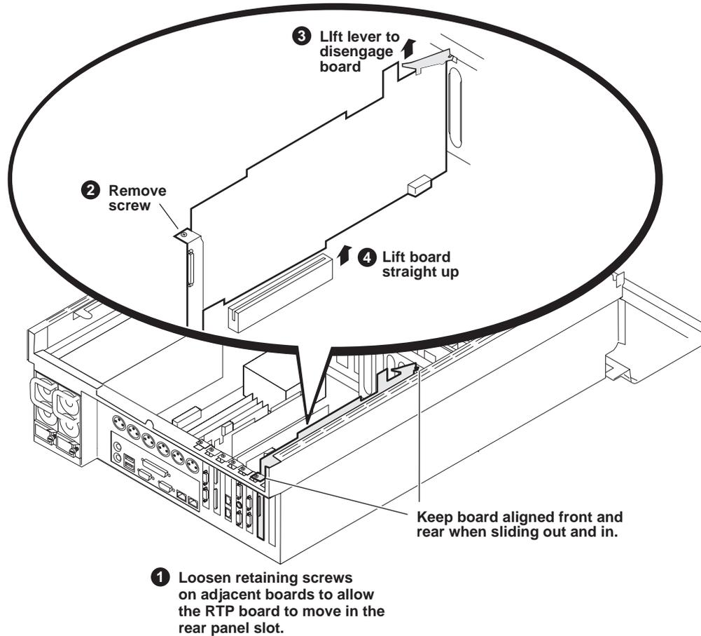
On HD/SD models the RTP board is in rear panel slot two, as shown. On SD-only models the RTP board is in rear panel slot five.
