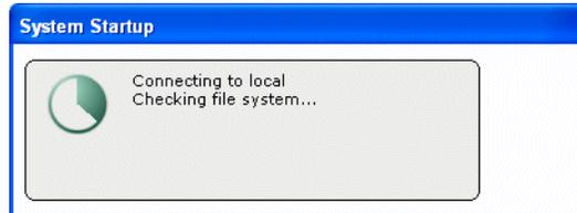
When all critical subsystem checks are successful, AppCenter workstation opens. If one of the system checks fails, a message appears and AppCenter does not open, so the K2 Media Client is unable to accomplish media operations. Refer to [“Critical system startup messages” on page 36](#) for a list of the messages that can appear.
