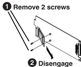
Use a #1 Phillips screwdriver to remove the screws.
