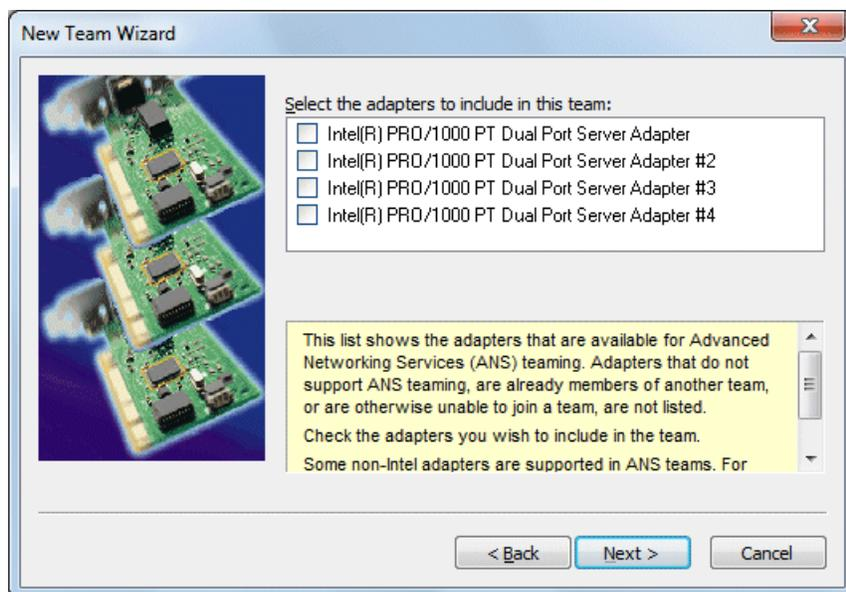
8. Select the check box for the adapter name that maps to Control Connection #1 and for the adapter name that maps to Control Connection #2. Click **Next**.
