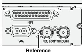
Through this hole a LED is visible. When the LED is lit, the reference signal is present and locked.
