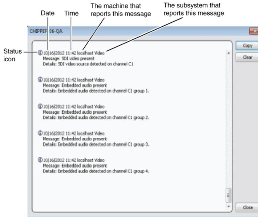
The StatusPane is used to view detailed system messages including status, warning, and error messages. System status messages provide status icons and a description of the status event reported by the message. If there is a problem, a corrective action is indicated. Use these messages along with troubleshooting problems to determine if a service procedure is necessary.
