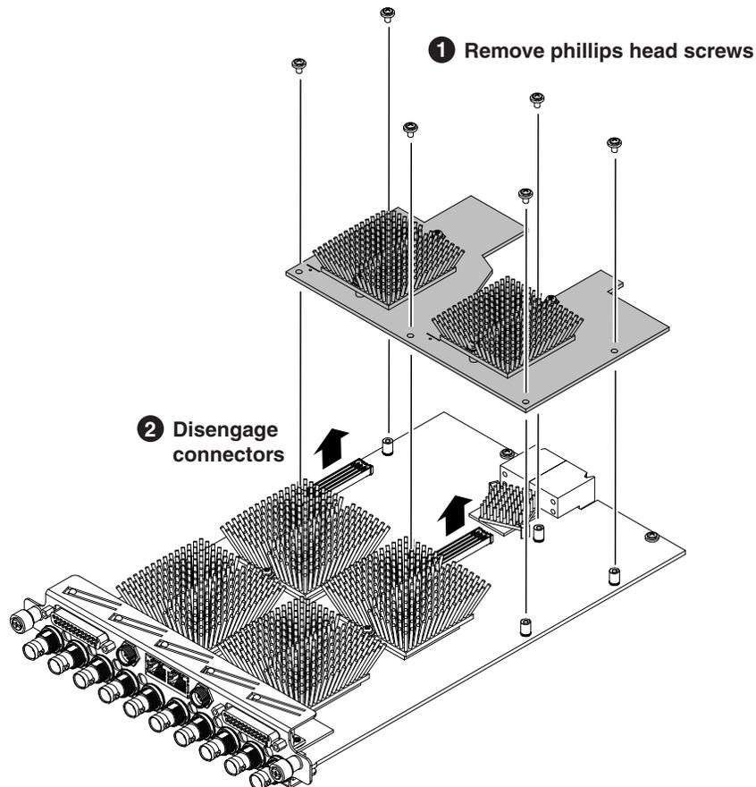
Use a #1 Phillips screwdriver to remove the screws.
