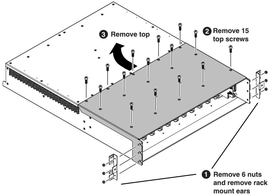
Use a #2 Phillips screw driver to remove the top screws.
