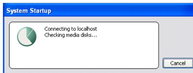
When all critical subsystem checks are successful, AppCenter opens. If a critical error occurs, a message appears and AppCenter does not open. You can check the list of the messages that can appear.
