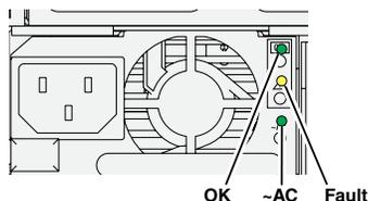
Interpret the power supply LEDs as follows:
