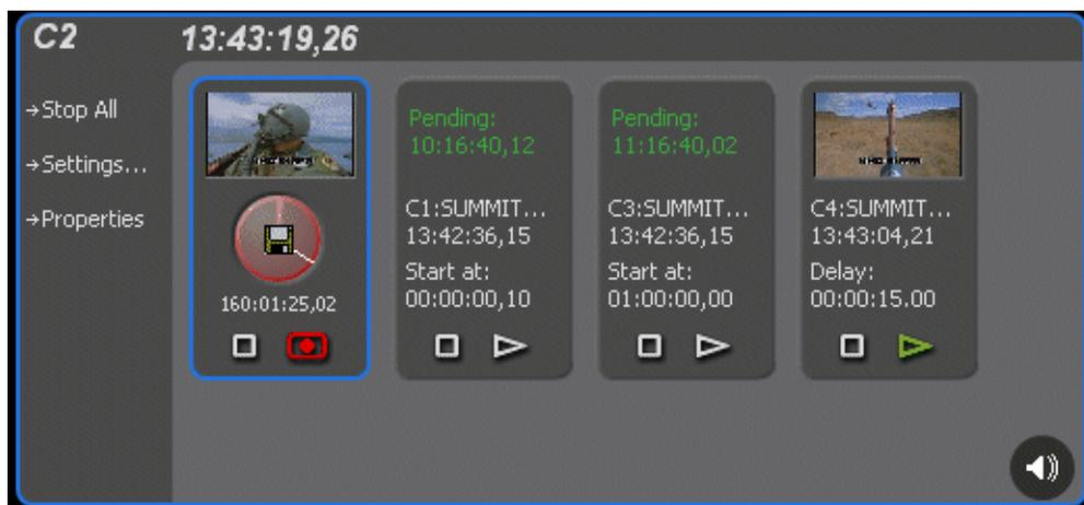
Note that the play channels used by this session of K2 TimeDelay do not show the TimeDelay application to their right. Instead, they show that the channel is in use by the TimeDelay application running on the corresponding record channel. Use the recording channel to interact with the TimeDelay application. In the monitor pane, a red outline indicates a recording channel and a green outline indicates a channel that is currently playing media.
