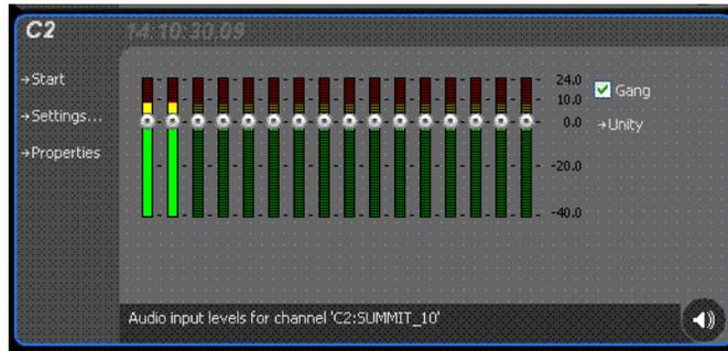
Each audio meter indicates the final (adjusted) audio level on the audio input or output for that track. A decibel scale is displayed alongside the sliders.
