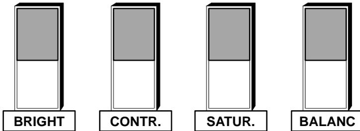
Bar graphs for the indication of the color parameters. The mask position is adjusted with four dipots.
