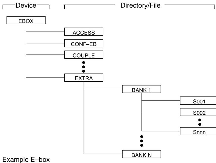
The highest level in the directory structure is the DEVICE level. Here all devices connected to the network (PANELS, E-BOX) are indicated. You can return to this highest level from any place within the directory hierarchy simply by pressing the **DEVICE** softkey (F19).
