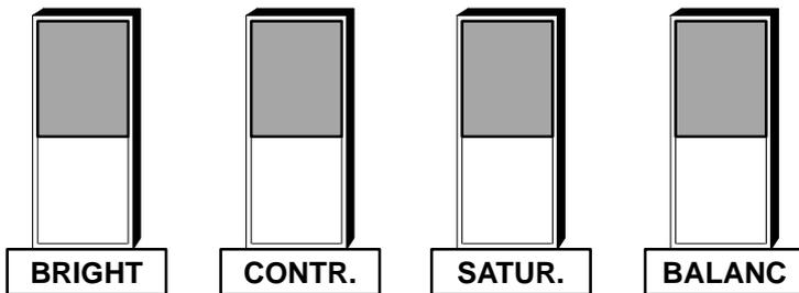
Bar graphs for the indication of the color parameters. These parameters are adjusted with four digipots.
