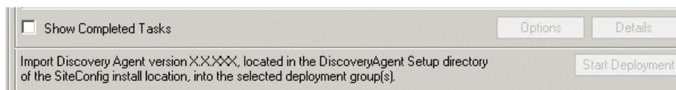
If a message instructs you to upgrade the Discovery Agent, on the control point PC go to the directory to which SiteConfig is installed, find the *DiscoveryAgent\_x.x.x.x.cab* file, add it to the deployment group, and deploy the Discovery Agent software as well.
