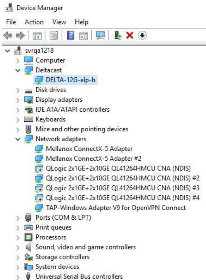
To check the version of drivers and firmware, right click on 'DELTA-12G-elp-h' and select 'Properties'. Select the 'Driver' tab in the window that appears. The number should be 6.19.13.0
